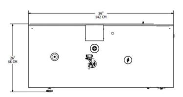
Note: Dimensions of WT-30LC shown. Outside dimensions for WT-30LC are the same as the WT-26.
